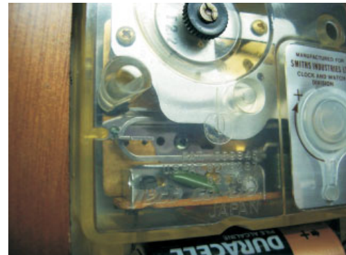
Ray's Smiths clock from the UK with a tuning fork driven movement made by JECO in Japan.
