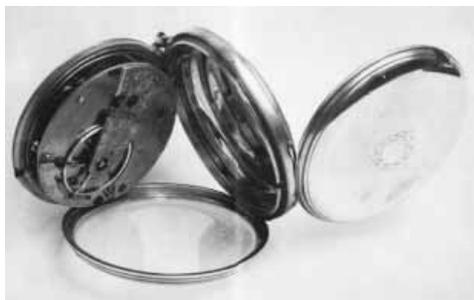
*English lever watch case construction. The glass opens to adjust the hands and the back door reveals the winding square.*
