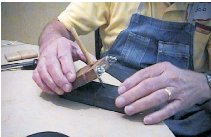
Bob Linkenhoker showed us provide a final polish to a graver using a home-made holder at our August meeting.
