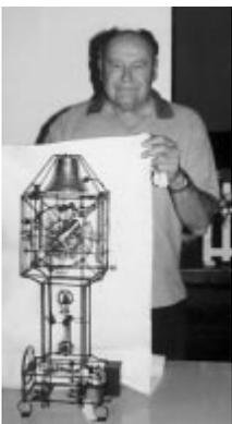
For the letter "K" Bud Sabien displayed a "crazy" electric-powered novelty skeleton clock. He likened it to one of Rube Goldberg's contraptions. Made mostly of welded rods, it featured funny little figures hanging on to the moving parts, and some novel gear and pinion construction. It's a real treat to watch, but a lousy timekeeper.
