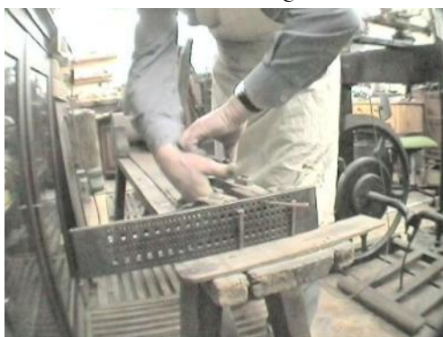
Tube making using Drawbench
