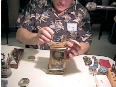
balance assembly by removing the screws that hold the platform down.
