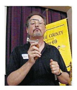
To place a blade in the saw, tighten the desired blade into the top clamp of the blade. Brace the top edge of the saw against your workbench. Place the handle against your chest and apply some pressure. You can now tighten the other end of the saw into the bottom clamp of the saw. Once you release the pressure you have applied to the saw, the blade will have sufficient tension for you to begin working.
