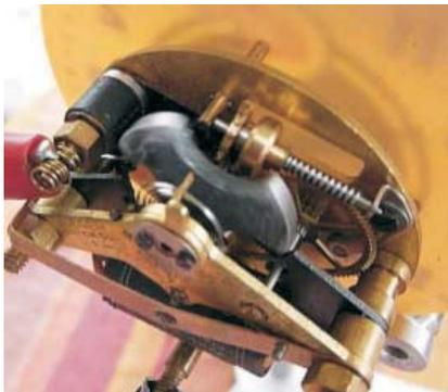
*Jaeger "Magnetric" movement showing three lobed balance wheel.*
