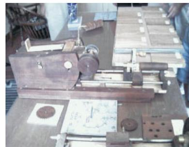
*Plate jigs & masks and an escape wheel cutting engine as used in the Porter contract technology.*
