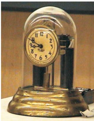
or five minutes thus small weights or small springs may be used. Also, since the weights/ springs are small, large gear reductions are not necessary and fewer wheels can be used thus the electric clock is a much simpler mechanism.
